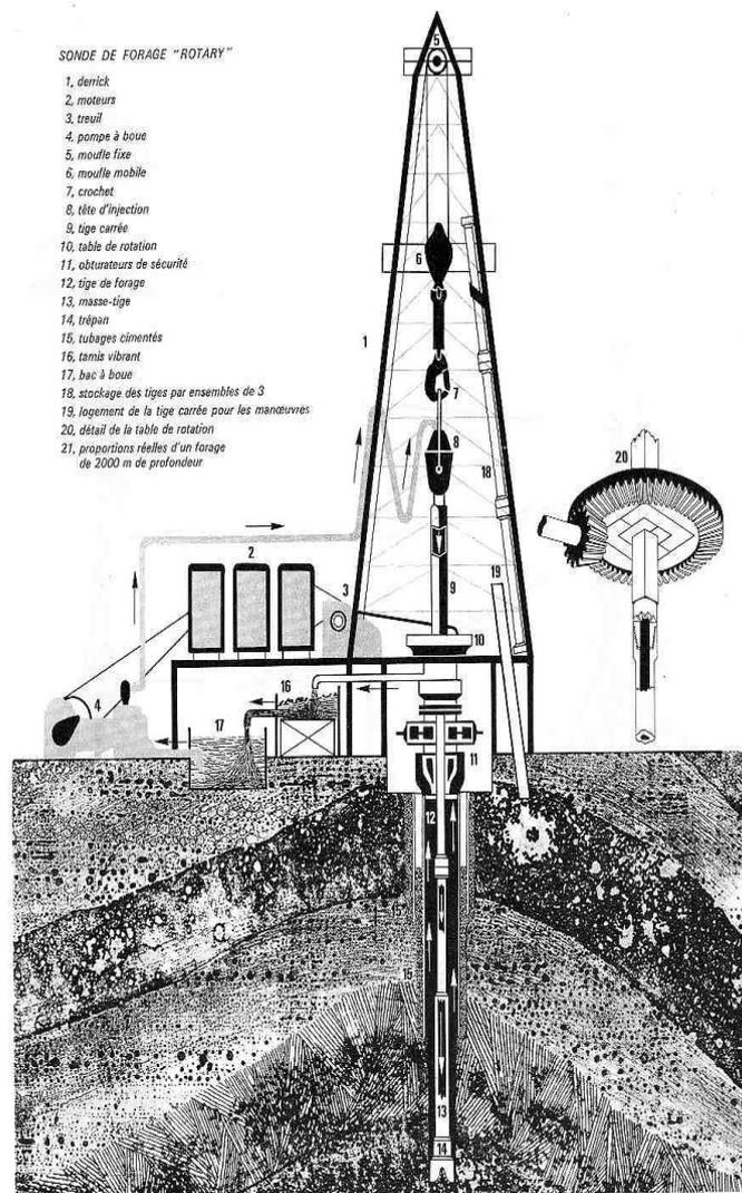
Figure 72: Sonde de forage rotary (document ENSPM)
